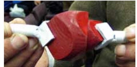
Roy used a piece of angle iron, cut so that when two pieces are joined by spot welding they form four faces of half a cube. A rod of appropriate dimensions (to be held in the jaws of a chuck and rotating centre) are then attached at the rear corner of each half-cube. Two opposite corners of the wood to be turned are fitted into these half-cubes, mounted on the lathe, then turned, as was described in the April issue of this newsletter.
