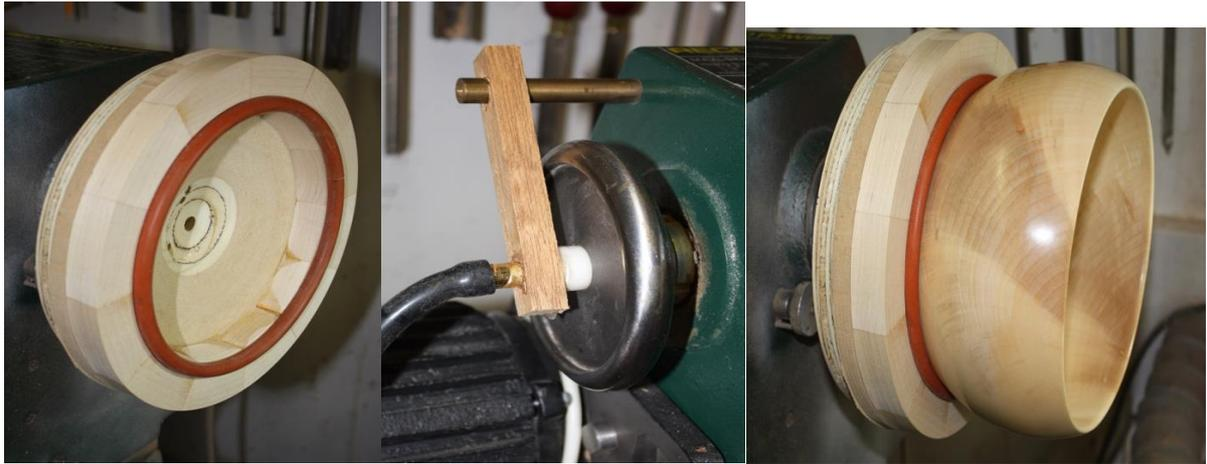
The photos show: the chuck mounted on the lathe via a face plate, the vacuum connection, a bowl mounted on the chuck.
